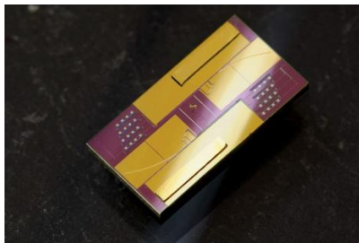
Fig. 6. Mid-IR tunable light source consisting of an SLED integrated on Thick-SOI. Chip size 5 \times 10 mm.
