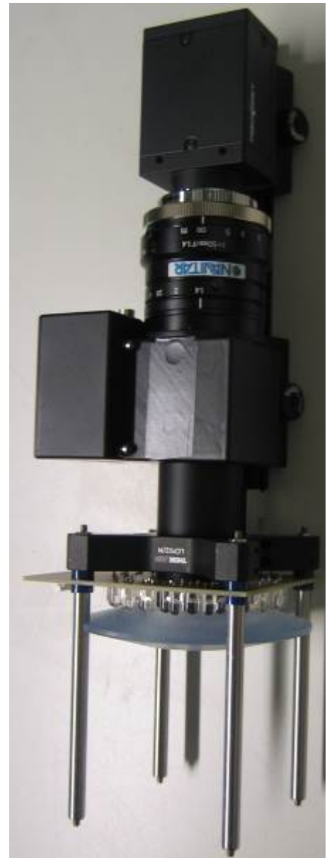
Fig 2. Hyperspectral imager laboratory prototype based on angle-tuned multi pass band filter, Leds and RGB image sensor.
